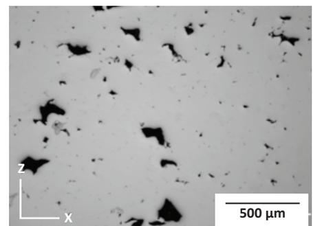
**Figure 4** - Optical micrograph demonstrating vapourisation porosity
