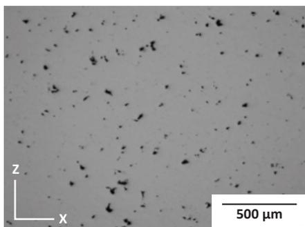
**Figure 2** - Optical micrograph demonstrating lack of fusion porosity
