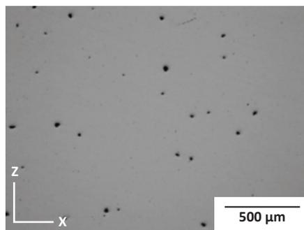
**Figure 3** - Optical micrograph demonstrating gas entrapment by insufficient overlap
