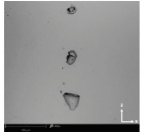
**Figure 5** - Optical micrographs showing vertical lines of porosity which align closely to crack initiation or propagation paths
