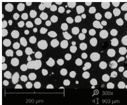
**Figure 1** - SEM Micrograph of mounted and cross sectioned LPW-718 powder
