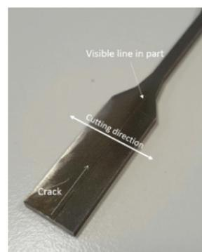
**Figure 7** - Photograph of block sample showing full width of crack and EDM wire cutting direction
